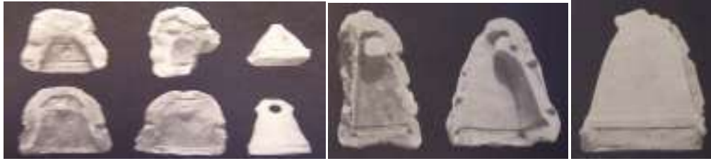
Fig.16 The plaster molds for casting bells and the two parts of the mold joined together After, Hickmann M.H.,(1949),nos.32312-14-15
