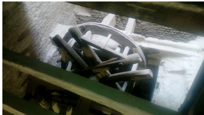
(Fig. 6) A water wheel that used to feed the palace with water in the past.
